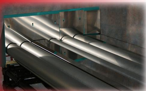
Our technologists studied the advantages and disadvantages of available systems and along with customer feedback, set out to design and develop the ultimate fibre feed control system. Lightweight, positively driven rollers replaced heavyweight belts.
