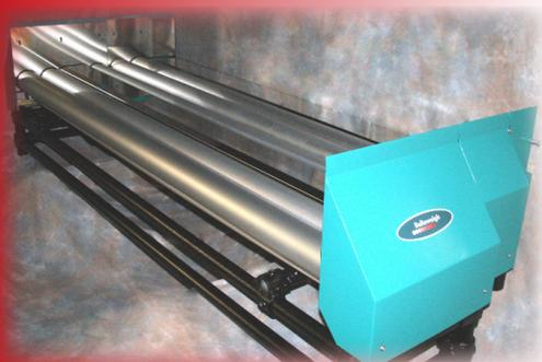
**Rollaweigh, the unique fibre feed control system from Garnett Controls has become a standard for quality and performance in card feeding internationally.**
